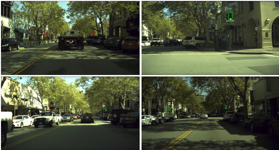
Fig. 8: Sample results. The color of the bounding box represents the classified traffic light state. The system can overcome hard false positives such as brake lights of a truck (top-left), however lamps can still yield false positives (bottom-left).
